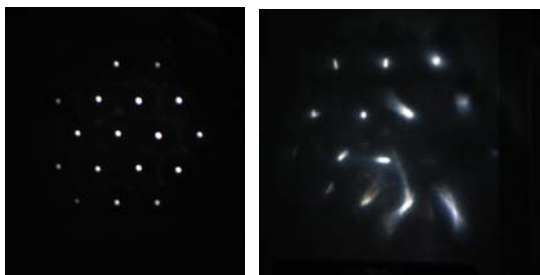
Figure 7. Light on the screen from the perfect eye model (left) and the aberrated (right).
