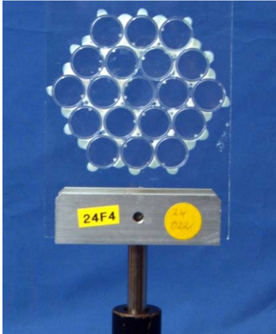
Figure 6. Lens array formed of a matrix of 16 lenses ( \text{\O} about 1.6 cm, f = 120\text{mm} ).
